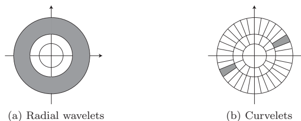
Figure 1.6 Tiling of the frequency domain by radial wavelets and curvelets.
