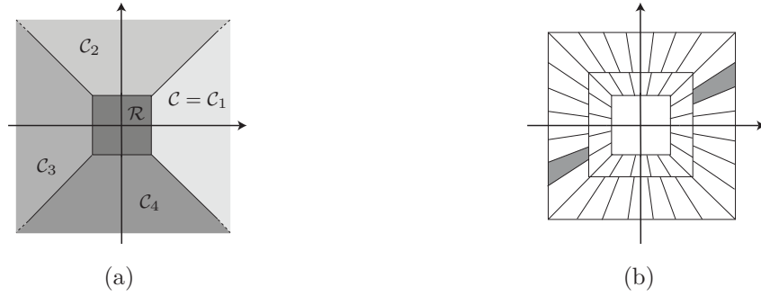
FIG. 1.2. (a) The cones \mathcal{C}_1 - \mathcal{C}_4 and the centered rectangle \mathcal{R} in frequency domain. (b) The tiling of the frequency domain induced by a (cone-adapted) shearlet system.
